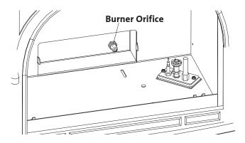
Figure 14. Change the Burner Orifice.
